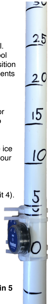
The HOBO Logger, strapped securely to the PVC pipe.
